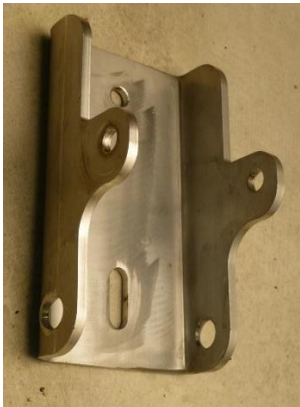
Mounting bracket with vertical anchorage points
